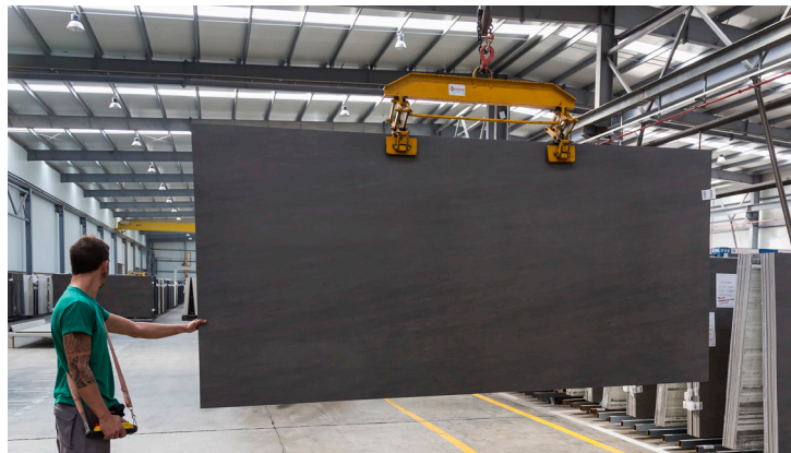
Image 2: Neolith slab handling with Clamp
